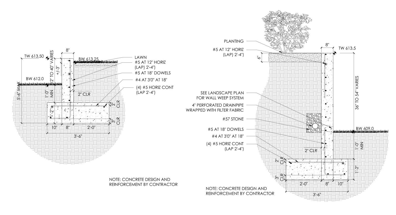
CONCRETE RETAINING WALL AT NORTH TERRACE SCALE: 3/4"=1'-0" L4.00
