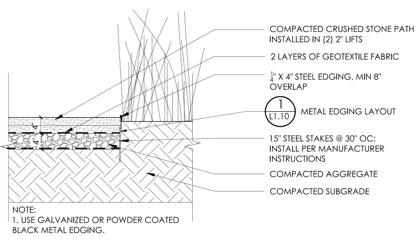
4 CRUSHED STONE WITH STEEL EDGING
