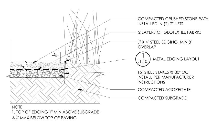
CRUSHED STONE WITH STEEL EDGING L4.00 | SCALE: 1"=1'-0"
