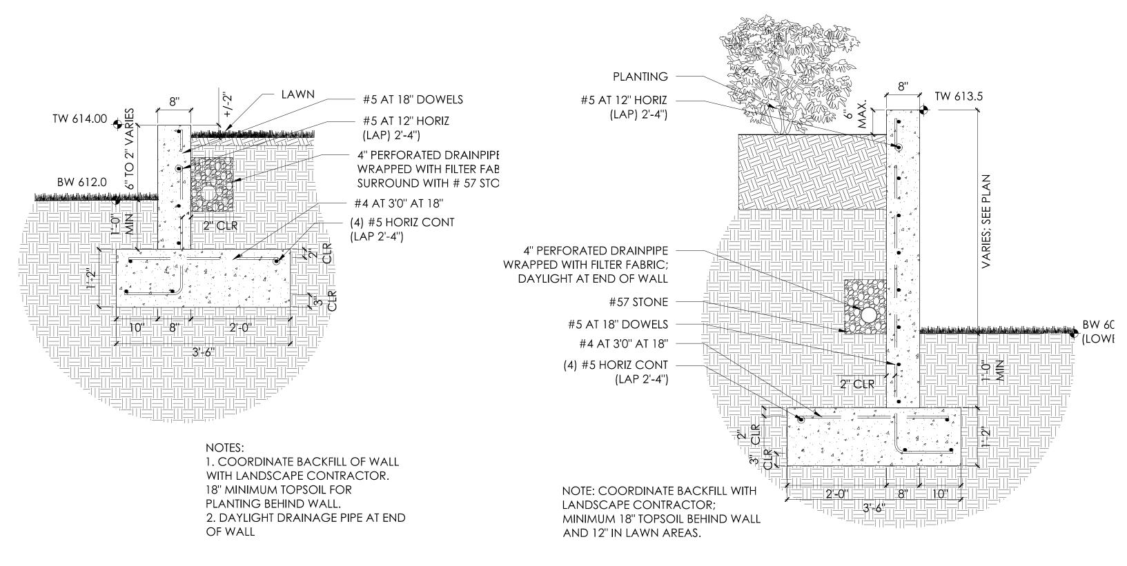
CONCRETE RETAINING WALL AT NORTH TERRACE
